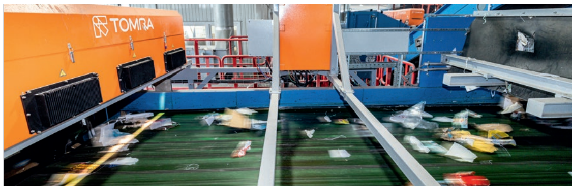
Keeping an eye on quality: near-infrared equipment identifies different materials based on the light they reflect
